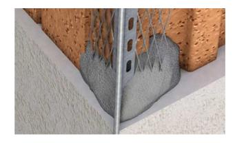
For plasterboard cladding, aluminium or plastic edge protectors can be used to great advantage to create the ideal corners, ensuring both correct and straight lines. They are also available in versions suitable for curved corners to facilitate the creation of unbroken and continuous curved edges.
